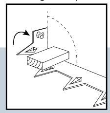
Use a workbench (if using a vice, use wooden blocks to prevent scratches) or a wooden block to bend the segments. Bend the segments by hand to create curved contours.
