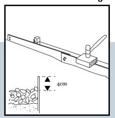
Tap the lawn edging segment gently down to the desired height of the border. For optimum stability, make sure that at least 4 cm is visible above the soil level.
