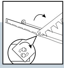
Insert the first segments loosely into the soil and connect the next segments one by one.
