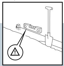
Mark out the desired contour (straight, curved, etc.) with twine and stakes. Dig a spade about 8 cm into the soil.
