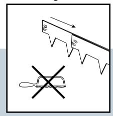
Sawing off excess length is not advisable. For optimum stability, let excess length overlap.
