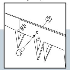
Another option is to secure overlapping segments by drilling a hole in them and securing them with a nut and bolt (of the same material as the lawn edging). For a coated finish, apply a primer to the materials to protect them from corrosion.
