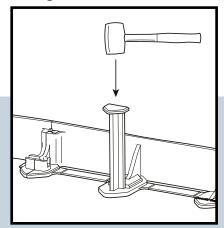
Use a hammer to tap the pegs carefully into the soil. Use all the pegs supplied to ensure the stability of the edging material.
