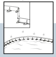
Insert the edging material in the right place. Slide the ends of the edging sections into each other to connect them. Any surplus length can be removed with a handsaw for wood.
