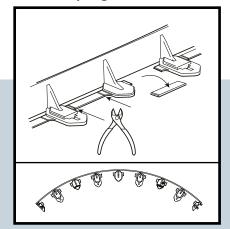
Use a wire cutter to remove the connecting pieces if making a curved contour.
